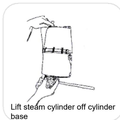
Lift steam cylinder off cylinder base
