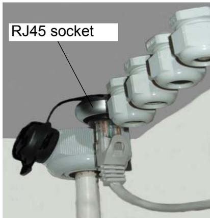
For connection of the Spa Touch Control to a HygroMatik steam generator a connection kit is required (see Section "Overview" last paragraph). One component part of this kit is an RJ45 socket in the form of a feedthrough housing (see adjacent illustration).
