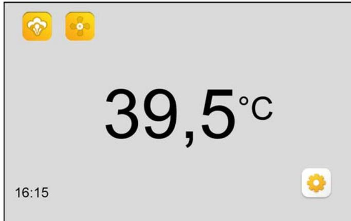
Steam release and fan are now enabled. By retouching the respective button the relevant function can be switched off although in the case of the steam release this is only possible as long as the operator has not set a default runtime.
